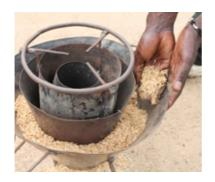
**4.** If the flame stops, new rice husk should be put in again to help the restarting process and air circulation should be ensured.
