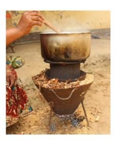
9. Supplementary fuels such as sawdust, small pieces of wood, dried coconut husks, peanut shells, corn cobs can be placed in an upright position in the inner drum or mixed with rice husk in the main drum. Add them in small quantities so avoiding smoke from the addition of too much fuel.
