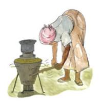
5. Grey ash eventually develops at the bottom of the centerpiece. When the rice husks inside the inner drum turn grey, tap the main drum with a stick to feed the flames again (approx. every 5-10 minutes).
