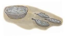
3. Insulate the inside of the basket by using a lining, stuffed with insulating material such as straw or hay, recycled clothing, foam rubber. Mazingira uses kapok.
